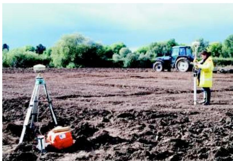
GPS base station positioned over an OS National Grid buried block (IS 100) in Field 7.
